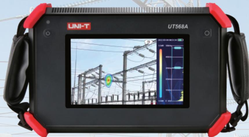
UT568A Acoustic Imager supports the ultrasonic frequency band. Through the combination of the sound source and video image, the constantly changing sound source distribution data is dynamically presented on the display screen, which is convenient for quickly identifying partial discharge phenomena and improving work efficiency.
